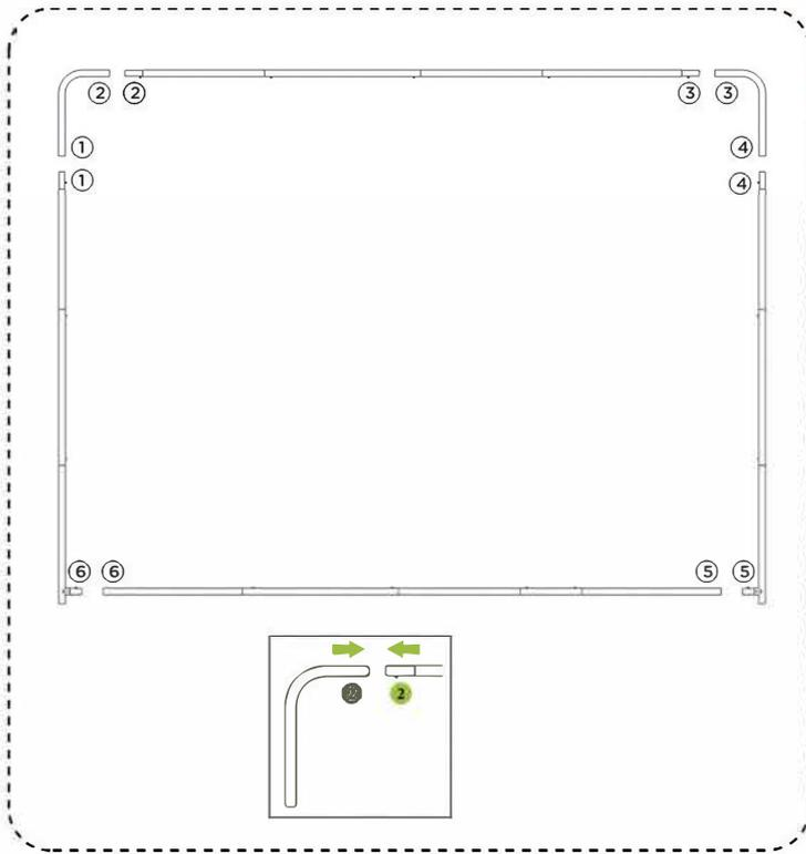
1 Connect tubes of the frame (there are number labels on tubes)
